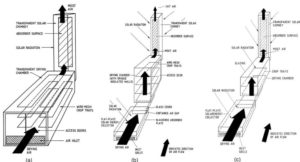
**Figure 2.** (a) Direct-type PSD, (b) indirect-type PSD, and (c) hybrid-type PSD (Ekechukwu, 1999).
