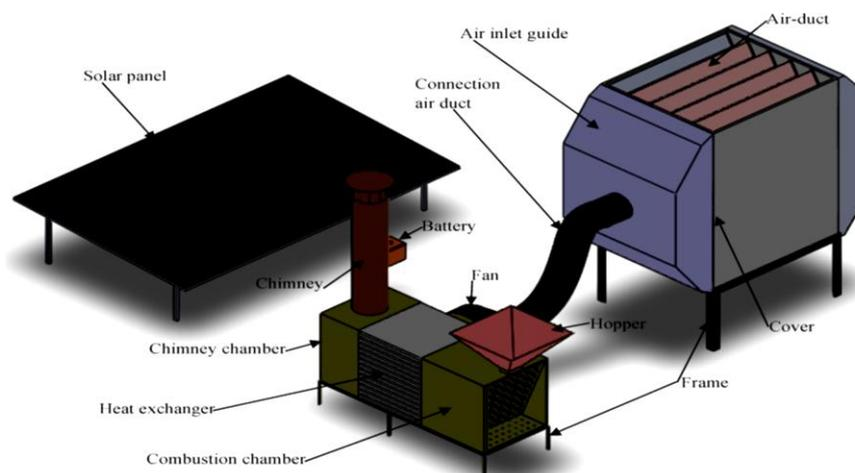
**Figure 5.** Novel mixed-flow rice dryer powered by rice husk energy (Mihret *et al.*, 2023).
