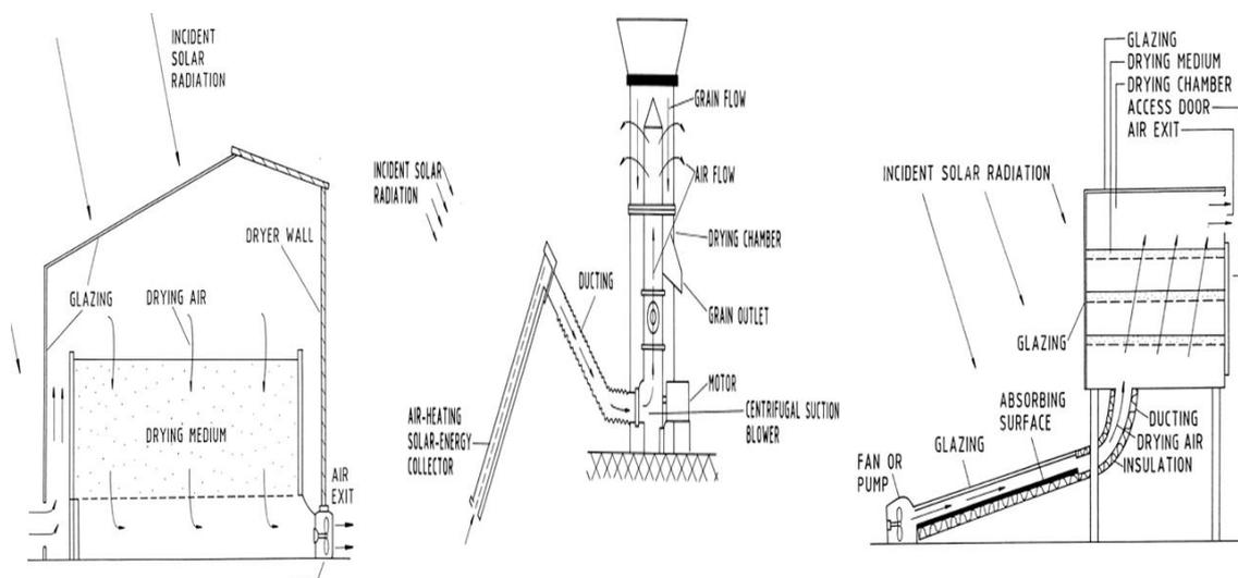
**Figure 3.** (a) Direct-type ASD, (b) indirect-type ASD, and (c) hybrid-type ASD (Ekechukwu, 1999).
